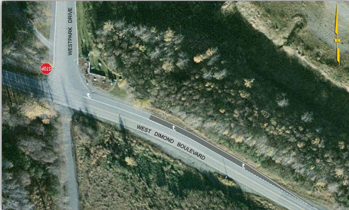
Figure 6.5 Right Turn Lane Extension At Westpark Drive
