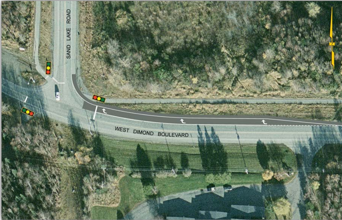
Figure 6.4 Signalized Intersection At Sand Lake Road Alternative
