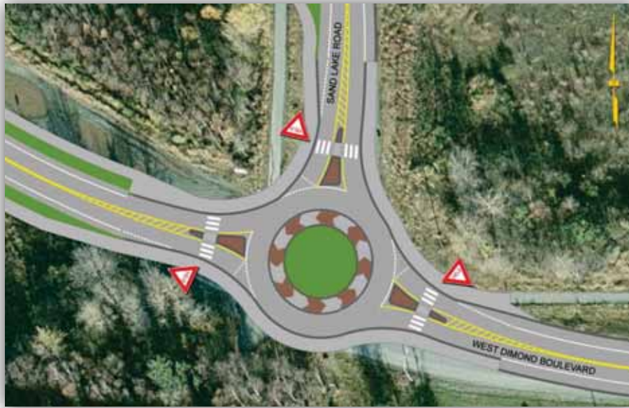
Figure 6.3 Single-Lane Modern Roundabout At Sand Lake Road
