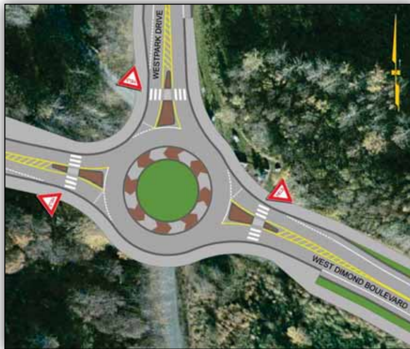
Recommended Alternative Single-Lane Roundabout at Westpark Drive Intersection
