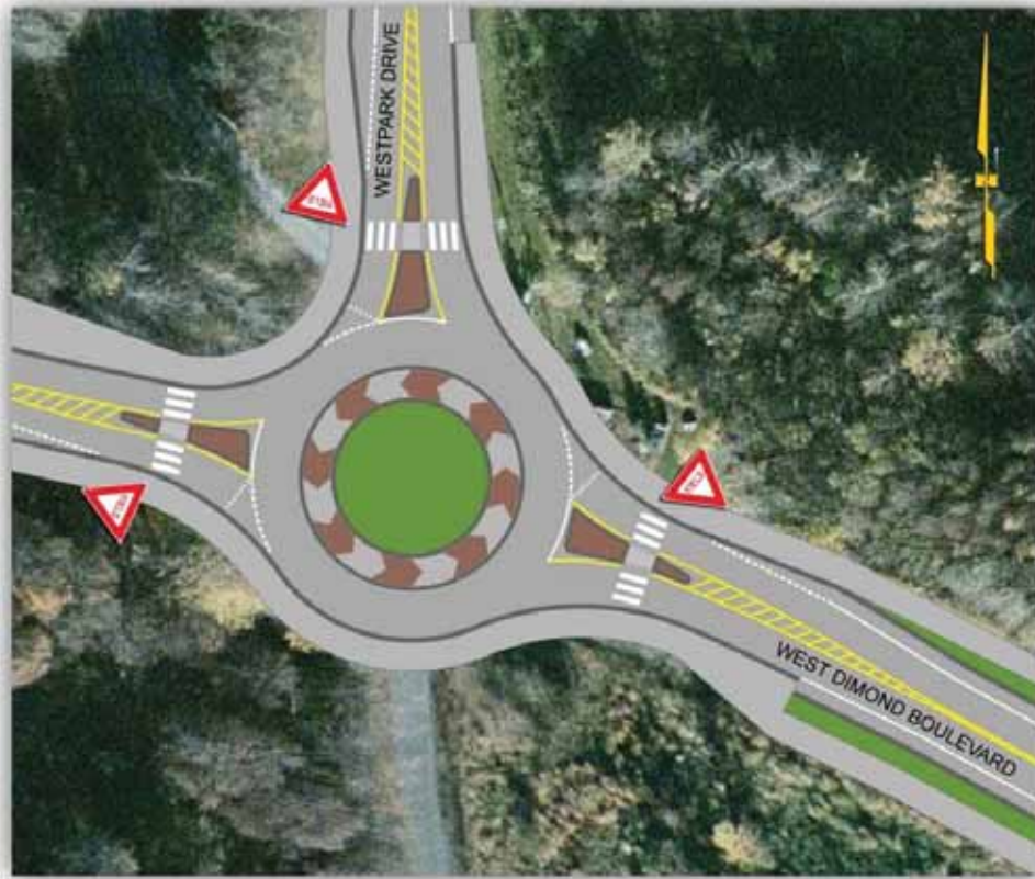
Figure 6.6 Single-Lane Modern Roundabout At Westpark Drive
